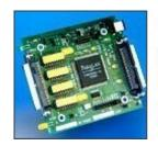
The board-level version Model MH17A is sized to fit in a standard 3.5" drive bay
