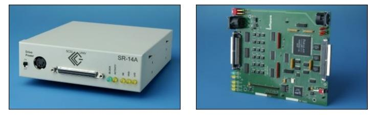
With the rigors of evidence standards in mind, hardware Write Blocking is a must. Paralan's SCSI Write Blocker allows data to be read at full speed, however, it will block any and all write commands thus preventing the possibility of writing to, or formatting the drive under examination. To prevent any system problems when write commands are ignored, a false acknowledge of writing is reported to the host computer.
